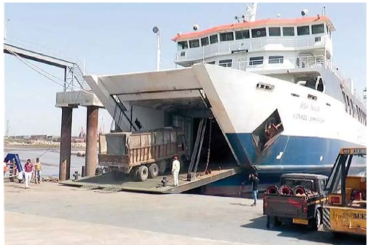
Typical RoRo ship in which vehicles and trucks with cargo can drive in and out.
