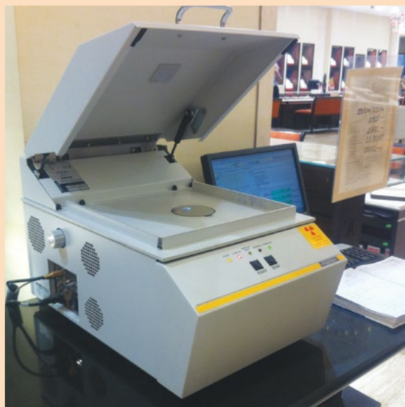
The Karat Meter- Used to test the purity of customer's old jewelry
