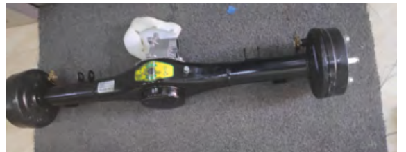
Differential and axlehub imported from China; costs Rs 2,500
