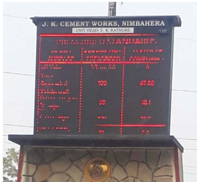
A live screen at the gate of the plant provides real-time emission readings of the plant and environment impact.
