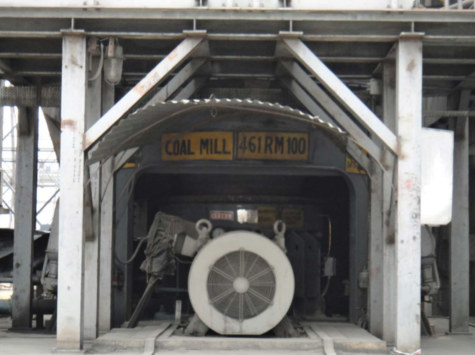
A grinding mill for coal used in the cement plant's captive-power generation.
