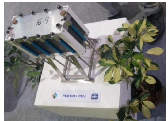
Hydrogen fuel cell developed by BHEL. Successfully tested for 10,000 hr
