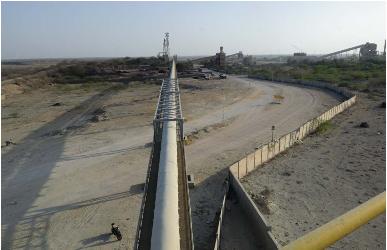
Conveyor belt laid from the mines to the plant as described by the Sanghi brothers to answer a question on incremental cost saving potential for first unit.
